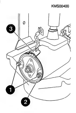
Disassembling stator frame and brush holder
